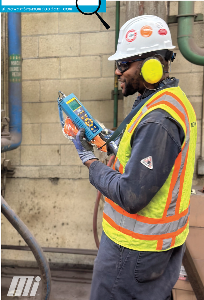
Figure 2 —As steam travels turbulently through the pipes, an ultrasound device can “hear” the movement of the steam, providing valuable insights into its flow and behavior. Image courtesy of Motion.
