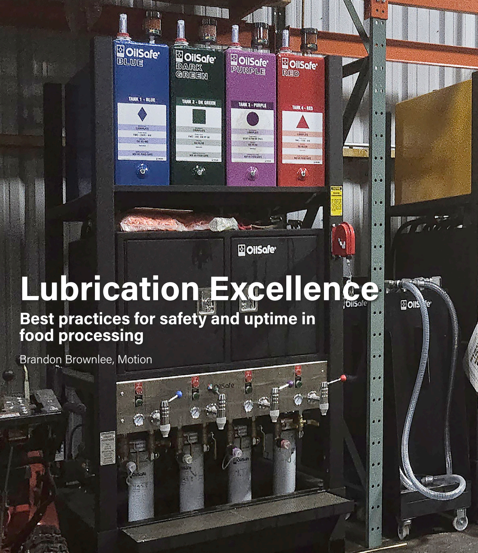
Figure 1—Use color codes and symbols to show which lubricant goes with each equipment piece. Image courtesy of Motion.
