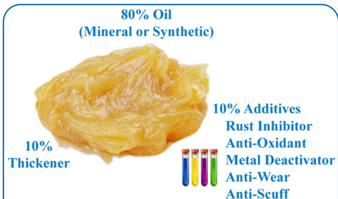
Figure 1 Diagram of grease composition (oil, thickener additive).
