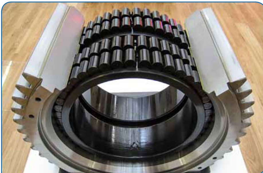
Black-oxidized wind turbine gearbox bearings: cylindrical roller bearings without outer ring, used in planetary wheels. (Photo courtesy SKF.)
