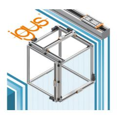
The heart of the new toothed belt axis is the linear guide system from the drylin W series, size 16, integrated into a robust, corrosion-resistant, clear anodized profile. Unlike other igus axes, the toothed belt runs inside the profile, giving the axis the appearance of a mechanical engineering profile.
