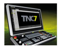
Heidenhain will also demonstrate the TNC7's component monitoring and process monitoring capabilities. Component monitoring can detect events such as tool breakage or excess force on the spindle. Process monitoring captures the data for a sample path and compares subsequent paths to this reference; deviations are graphically displayed, so operators can pinpoint the location.
