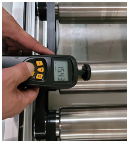
An instrument measures the performance of conveyor rollers driven by Eagle Poly-V belts, which maintain consistent tension and immediately transmit the motor's action to the rollers, unlike traditional roller chains.
