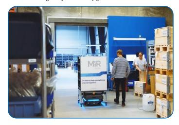
With five autonomous mobile robots, MiR has the widest range of AMRs in the market to take over various transportation tasks, from moving smaller parts to heavy duty loads up to 2200 pounds (1000kg). The largest robots can automatically pick up, transport and deliver pallets. Regardless of the task, these collaborative AMRs are designed to work alongside human colleagues and relieve them of various physically strenuous work so they can focus on more valuable tasks.
