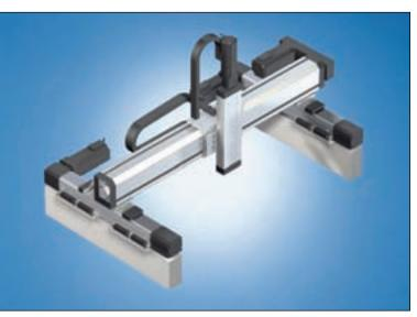
The BKK and BKR Bridge Modules are an expansion of Rexroth's linear modules. The aluminum extruded profile provides high torque stiffness to reduce deflection where the module is not completely supported. Y axes for gantry systems are an example of this where the bridge modules replace the configuration of parallel linear modules.
