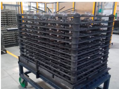
Figure 6—Load of sliding gears (CFC-fixture consisting of 12 layers).
