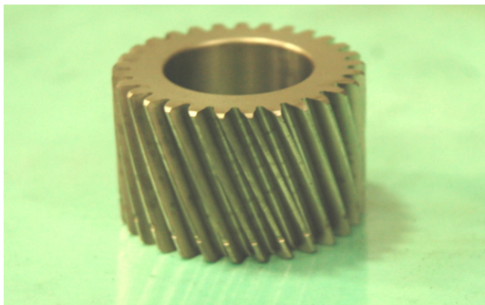
Figure 15—Final-drive pinion planetary gear (diameter = 31 mm, 24 teeth).
