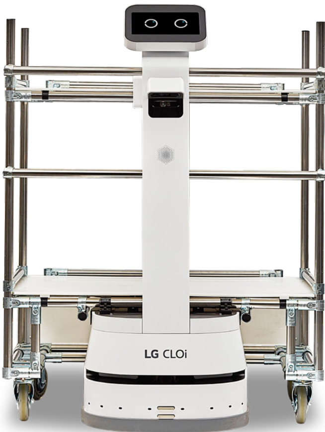
LG CLOi CarryBot is an autonomous mobile robot (AMR).
