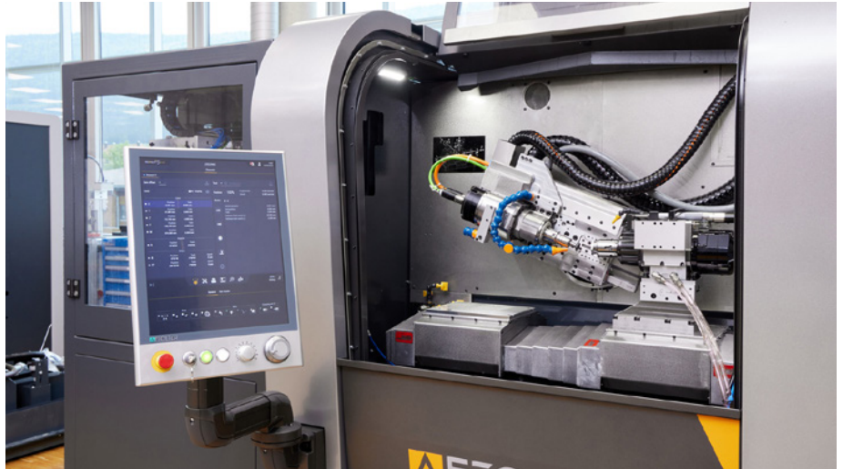
Different CNC machine, same control core: Affolter synchronizes three high-speed spindles with PC-based control from Beckhoff in its own machining centers.
