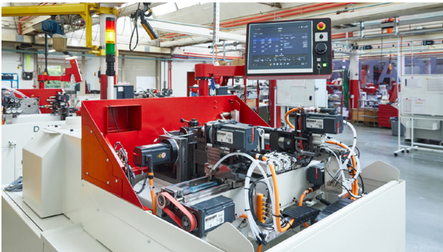
Esco relies on a control solution based on TwinCAT CNC developed by the Swiss Beckhoff Solution Provider Affolter across all machine series.
