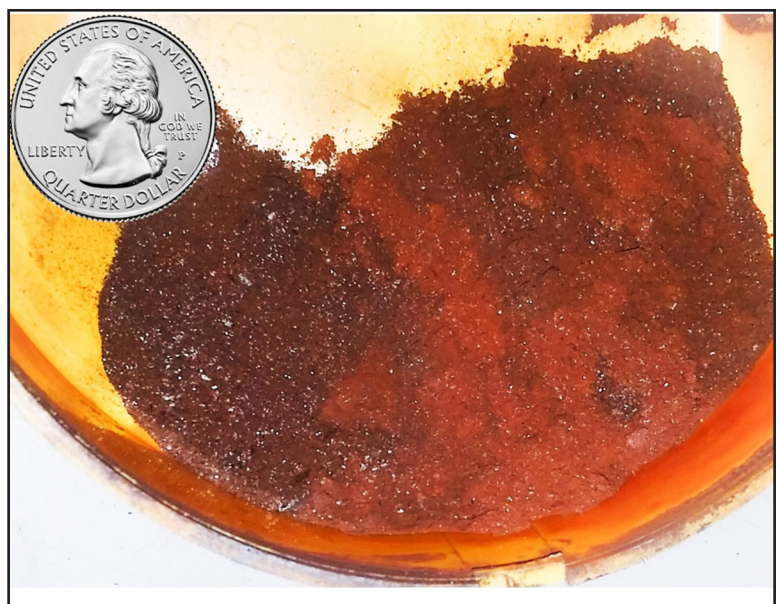
Figure 3 Fine oxide powder as a result of fretting.
