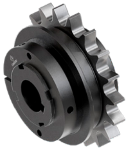
The EDF/F series is a ball torque limiter, which consists of two halves: a driving member and a driven member that are separated by a set of steel balls housed in grooves on both members.
