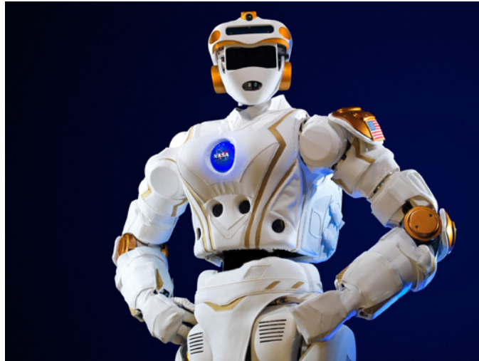
Valkyrie robot equipped with series elastic actuators (SEAs). Valkyrie specifically has five series-elastic rotary actuators and two linear actuators in the arms. Six finger and thumb actuators. Five series-elastic rotary actuators in the upper leg and two in the ankles. Five series elastic rotary actuators in the torso.
