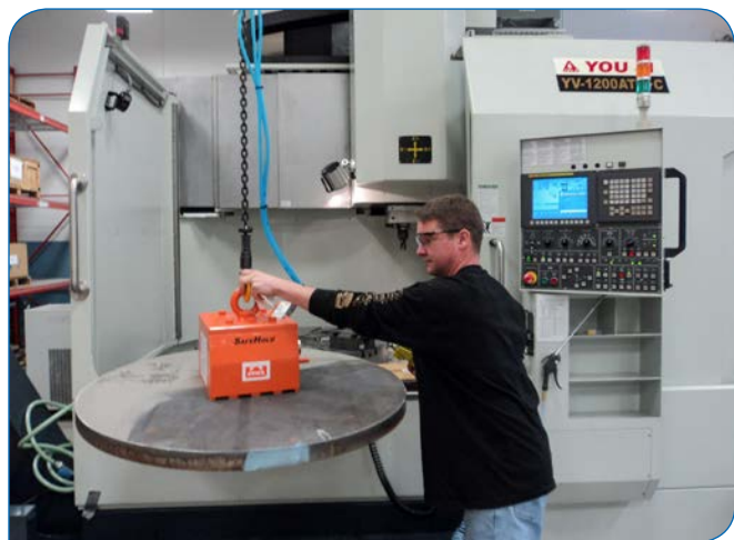
A production supervisor from KTR Corporation loads a large brake disc onto the vertical lathe machine.
