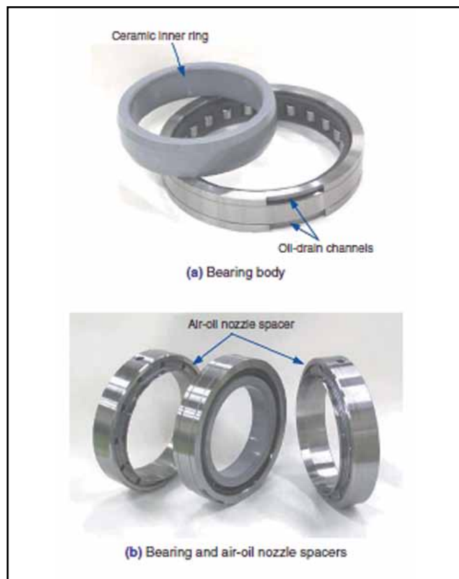
Figure 13—Developed, NU-type cylindrical roller bearing.
