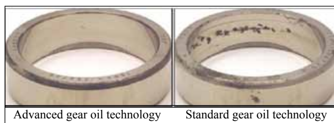
Figure 13—Emcor rust test with 0.5% NaCl water.
