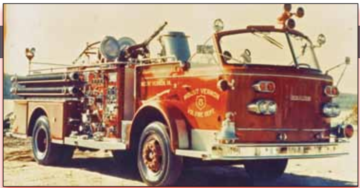
A 1961, 900-Series American-LaFrance 1,000-gpm pumper truck. The engine is by Boeing—a $10,000 option. The truck was one of three that American-LaFrance built that year and the only one shipped to the East Coast—specifically, to Mount Vernon, Virginia, where Dave Collins worked at the time as a professional firefighter. Note how the clearance between the top of the tire and the front fender opening speaks to how light the engine was. (courtesy Dave Collins).
