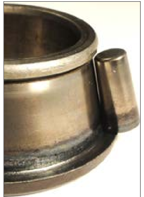
Photo 2 TRB run with no lubrication.
