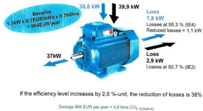
Figure 4 The various losses and motor efficiency of the ABB 50 hp (37 Kw) induction motor in black; and the equivalent SynRM motor in blue.
