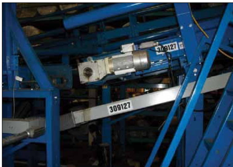
Figure 7—Example of a rigid-mounted installation; the bolt through the mounting plate prevents run-out of the driven shaft, resulting in all of the run-out of the shaft transferring into the unit—causing seal and/or bearing failure.
