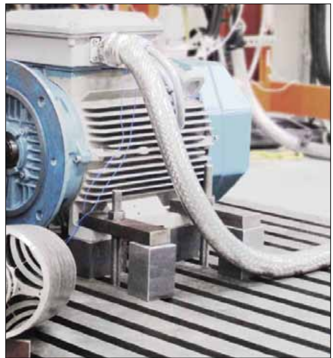
Figure 2—The possibility of high-speed operation helps to eliminate mechanical power transmission elements, such as gearboxes.
