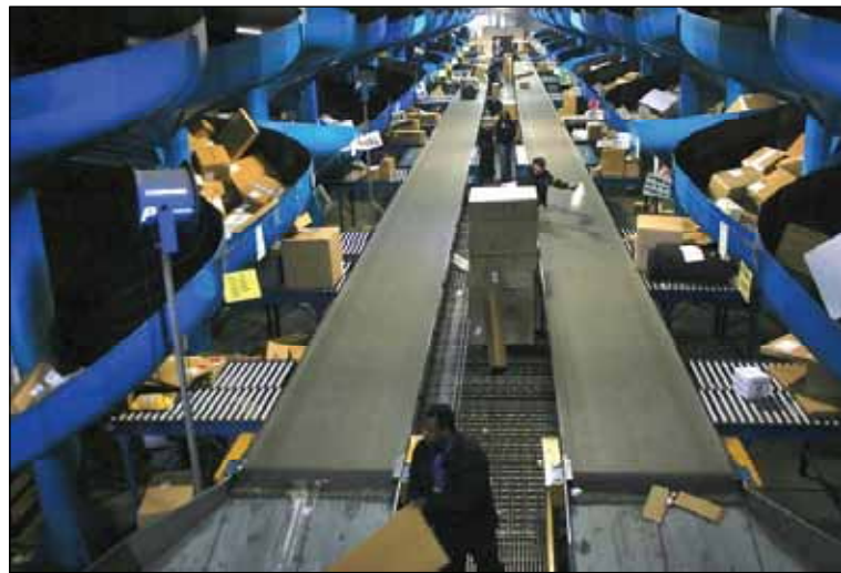
Figure 3—Main feed belts.
