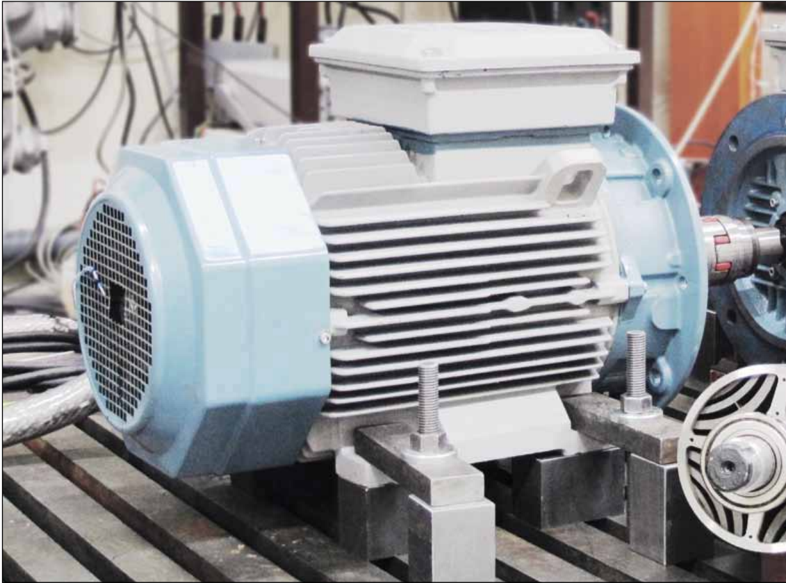
Figure 1—A motor-and-drive system undergoing highly accelerated stress testing (HAST). (The above and all other pictures/images courtesy ABB).
