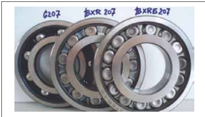
Figure 13—Deep-groove ball bearing 6207 with 9 balls; ball roller bearing BXR 207 with 11 rollers; ball roller bearing BXRE 207 with 14 rollers.
