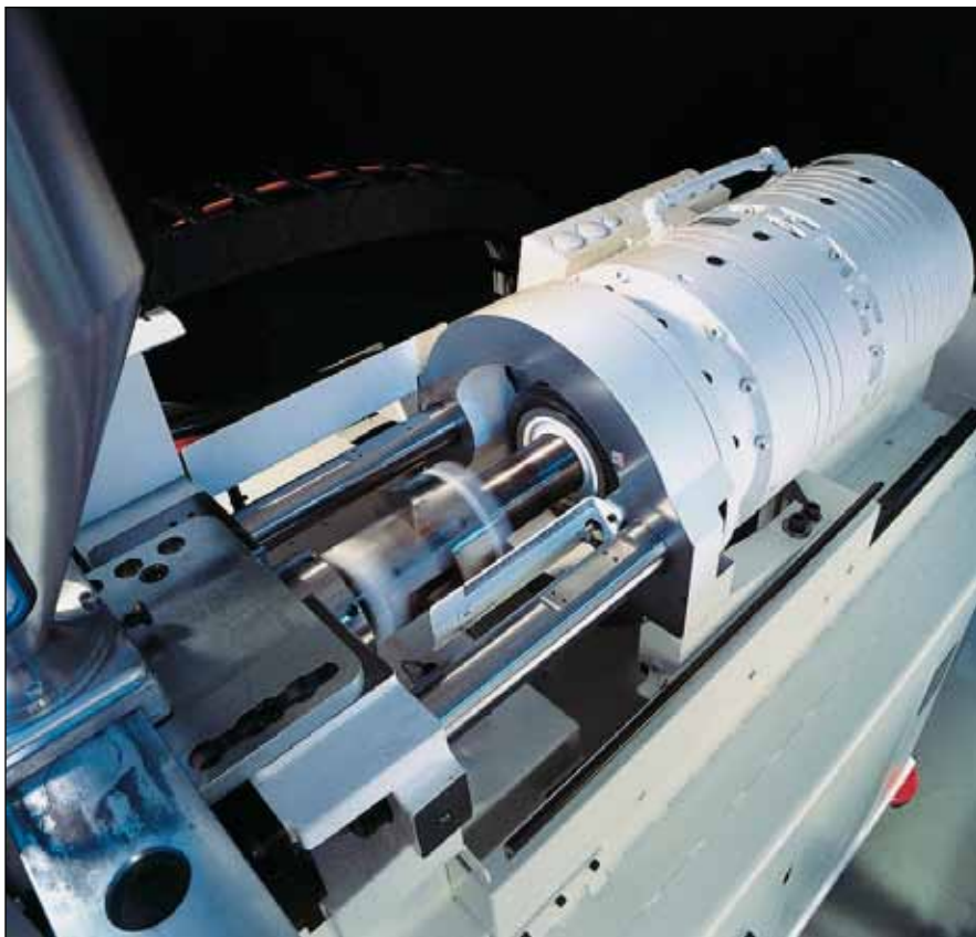
Hollow-shaft torque motors are used in a wide variety of machinery.
