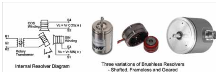
Figure 5—Diagram and examples of resolvers.
