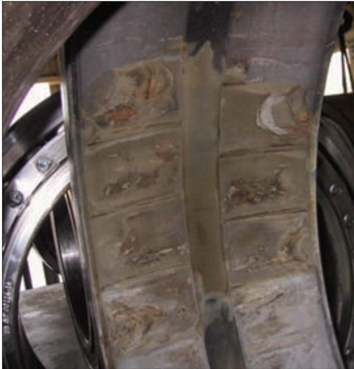
The outer race of a spherical roller bearing in need of bearing remanufacture.
