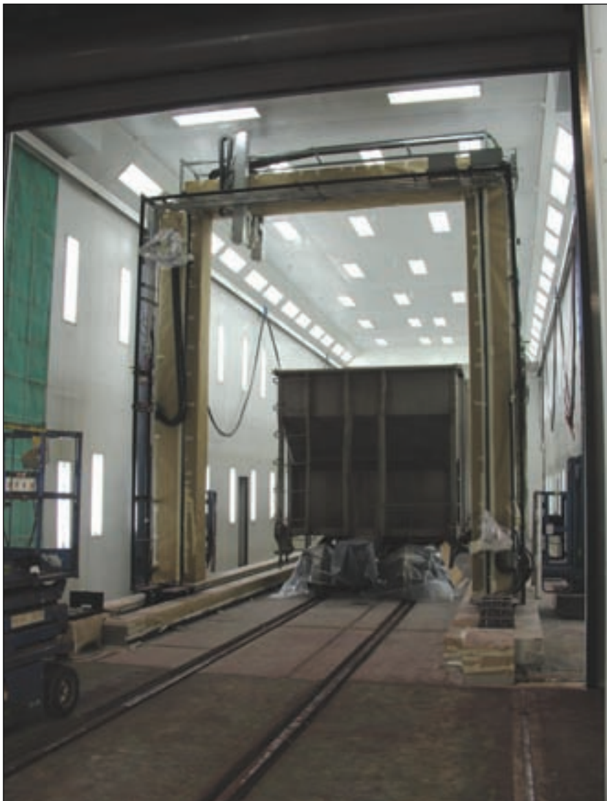
This automatic boxcar painter uses bearings from Lee Linear.
