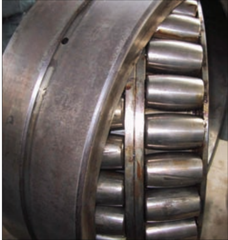
A large spherical roller bearing and outer race showing the condition of a bearing in need of bearing repair services.
