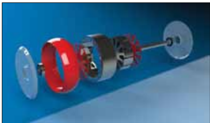
Figure 4—An exploded view of the mechanical design of our wheel motor.
