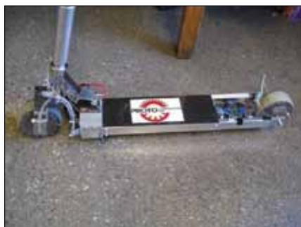
Figure 10—The assembled scooter with two motors installed.
