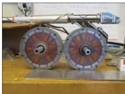
Figure 9—The rear motor (left) and front motor (right) differ only in the number of turns-per-phase.
