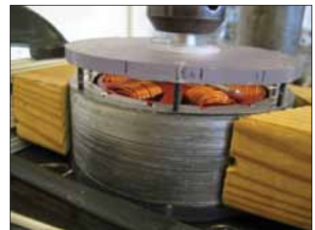
Figure 7—The stator and second side plate are dropped into the rotor with the aid of a drill press.
