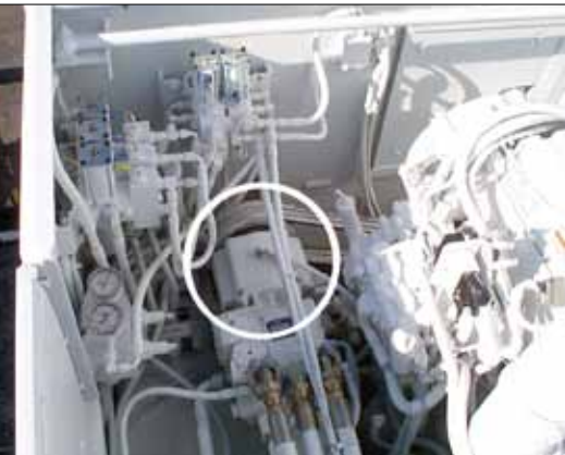
The hydraulic pump motor is connected to Zero-Max Overhung Load Adaptors.
