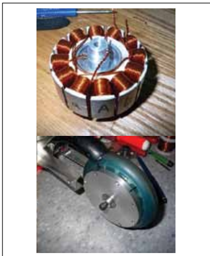
Figure 3—A kick-scooter wheel motor built by MIT student Charles Guan.
