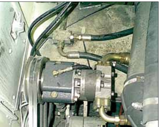
The adaptors used in the Roadtec system have a special oil drain port to facilitate lubrication.
