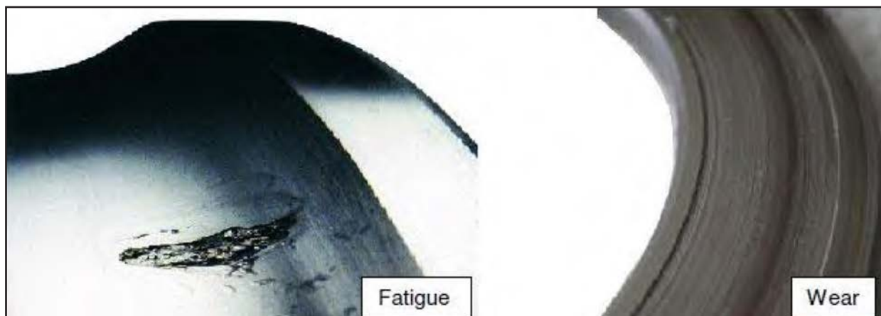
Figure 5 Example: typical rolling bearing failures.
