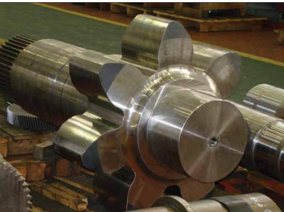
The final drive/output pinion for the jacking gearbox provides the power needed to operate the platforms in harsh conditions (courtesy of SKF).
