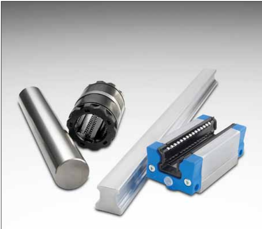
The two major types of linear guides are round rail bushing bearings and profile rail bearings. Round rail ball bushing bearing systems accommodate torsional misalignment caused by inaccuracies in carriage or base machining or machine deflection with little increase in stress to the bearing components. Profile or square rail systems offer higher accuracy, higher rigidity, higher load-life capacity and are also very compact.
