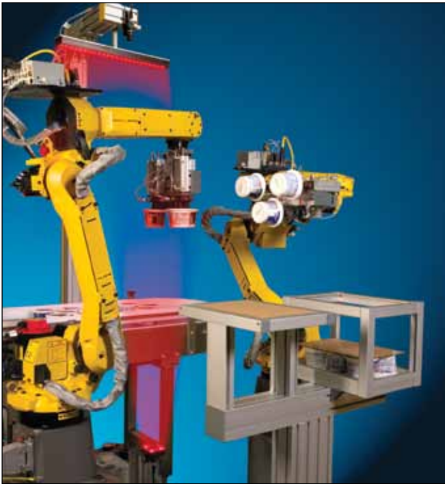
An M-101A robotic unit demonstrates material handling for the food and consumer goods industry (courtesy of FANUC).
