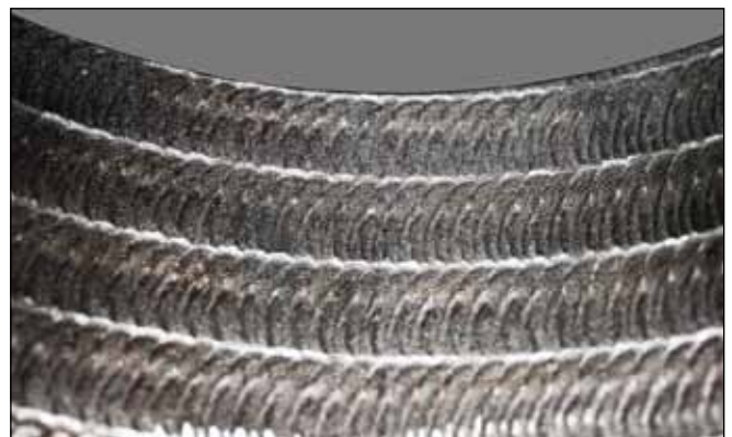
Arc welding with oscillation creates a pipe overlay of wider stringer beads.
