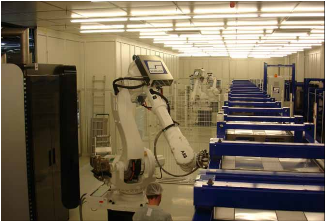
ABB Robotics gripper design enables a robot to handle the complete cutting process in solar modules (courtesy of ABB).
