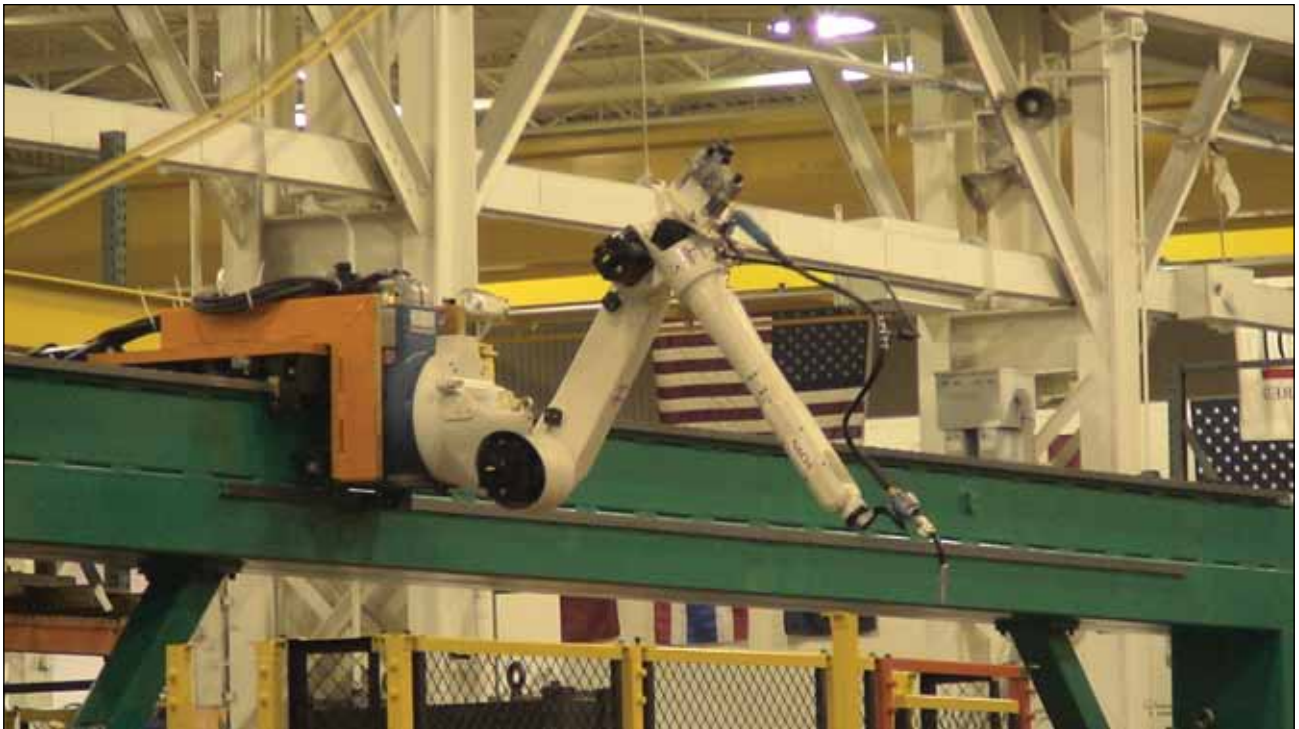
This Nachi MV06-L Robot is horizontally mounted on a traversing servo driven slide unit (courtesy of Nachi Robotics).
