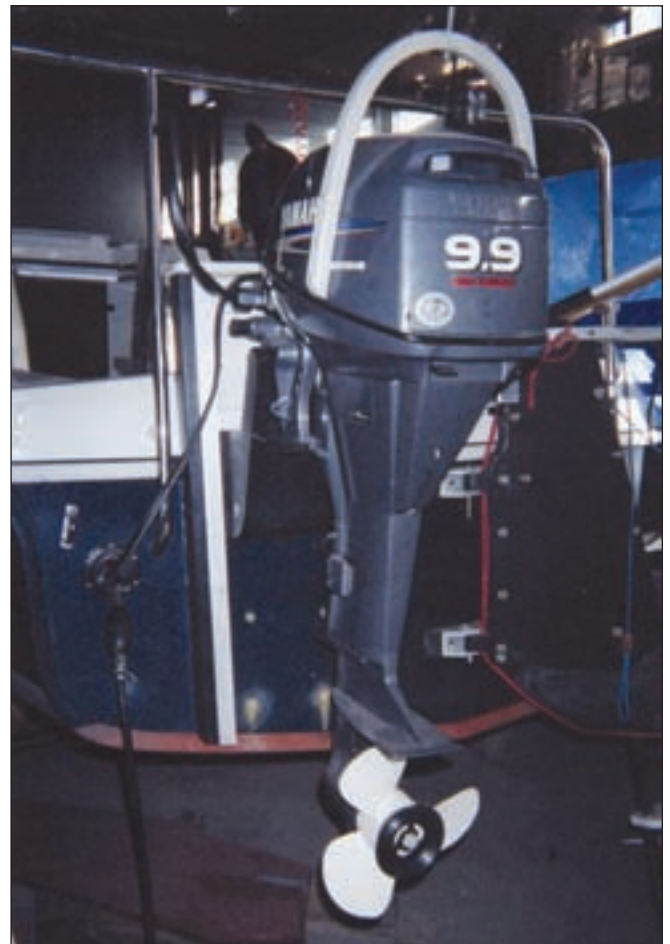
The Rhodes 22 is equipped with a mechanism that lifts an outboard motor in vertical movements.
