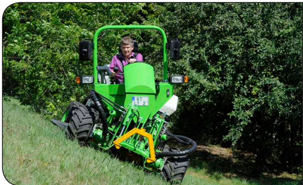
The LinsiTrak’s operator sits vertically in the seat even on a 45 degree slope (all photos courtesy of Bosch Rexroth).
