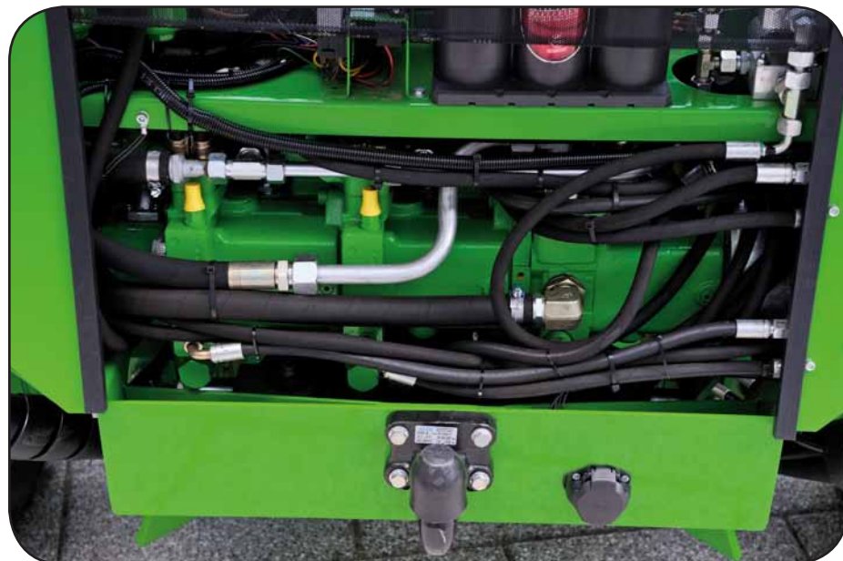
All three A10VG adjustable pumps used in the LinsiTrak are at a common location.
