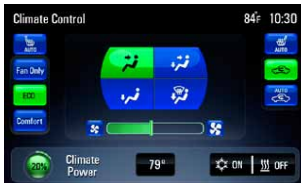
2011 Chevrolet Volt Climate Control screen: Volt owners can control the in-vehicle climate through the Volt's center stack 7-inch LCD touch screen.
