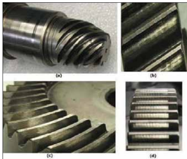
Figure 7—Hyponic gear components after 2.5 million cycles: a) hypoid pinion; b) spur gear; c) hypoid gear; d) spur gear pinion (Ref. 2).
